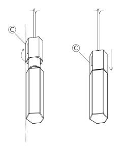
STEP 7 Rotate metal steeve ⑦ To align with the bulb
